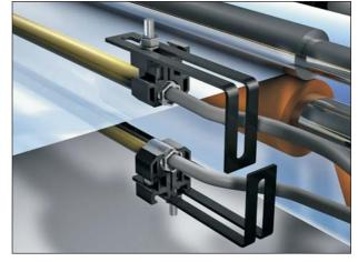
The material web brings along additional electrostatic charge from the machine. With the ionizing bars El VS in front of the roll the level of static charge can be lowered to a minimum. Fixation possibilities with different types of brackets and bar holders (photos 4 and 5) enable the installation for any machine construction.
