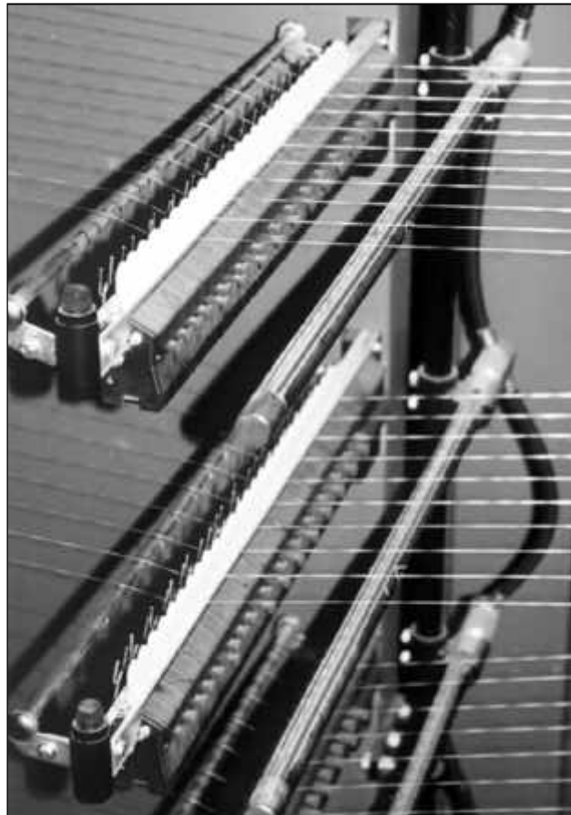
Photo 2: Special ionization system for bobbin and warp creels
